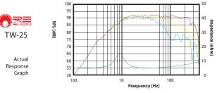
The frequency responses above show measured free field sound pressure in 1, 30, and 60 degrees, mounted in a 0.6m by 0.8m baffle. Input 2.83 Yms, microphone distance 0.5m, normalized to SPL 1m. The impedance is measured without baffle using a 2V sine signal.
